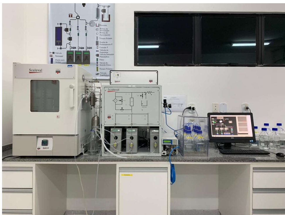
Figura 17: Tube bloking test (TBT). Scalavel, fabricado pela VINCI Technologies.
