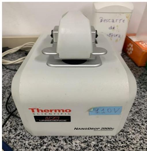
FIGURA 2. Equipamento NanoDrop 2000c (Thermo Scientific)
