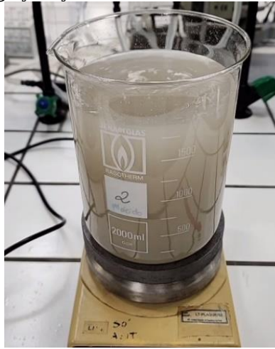
Figure 1. Water agitation with gray clay to prepare synthetic water.
