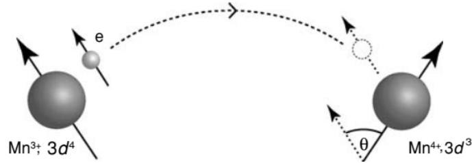
Figure II.1: The double-exchange interaction: An electron preserves its spin orientation as it hops between adjacent localized ion cores, mediating ferromagnetic alignment. adapte from [4]
