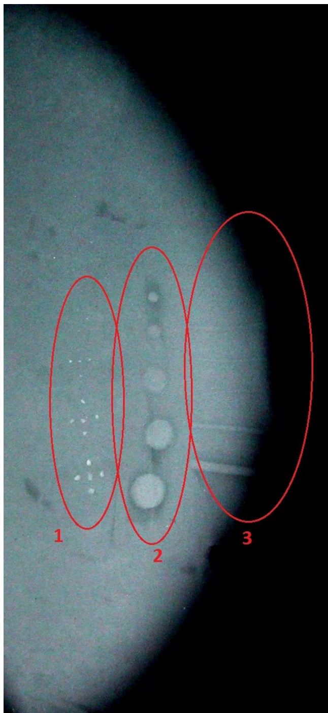
FIG. 4. Image of the base material containing inserted artifacts: microcalcifications (detail 1), tumor masses (detail 2) and fibers (detail 3).
