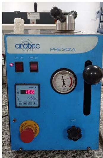
**Figura 1: Embutidora AROTEC PRE 30Mi<sup>®</sup>**
