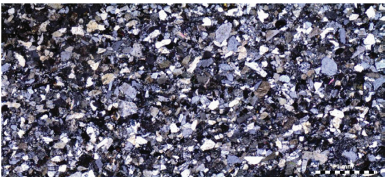
Figure 5. Overview of the section of sample C, showing the equigranular structure, absence of a tectonic matrix, and no grain alignment.
