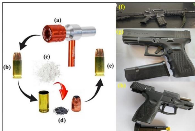
Fig. 2. Marker ammunition insertion and the weapons employed in the forensic tests. Caption (a) inertia hammer used to disassemble all the ammunitions; (b) 9 mm ammunition; (c) luminescent compound (not irradiated with U.V light); (d) disassembled ammunition with the compound added to the ammunition load; (e) closing of the marked ammunition; (f) Taurus® T4 rifle, 5.56 mm; (g) Glock® 23 Gen4 pistol, 0.40 S&W; and (h) Taurus® G2C pistol, 9 mm.
