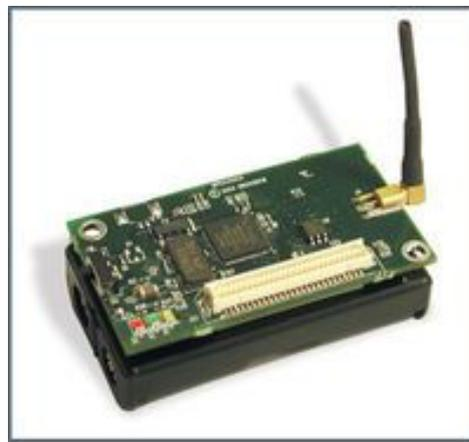
Figura 5.3: Sensor MicaZ com processador AVR Atmega128 (LORINCZ, 2006).
