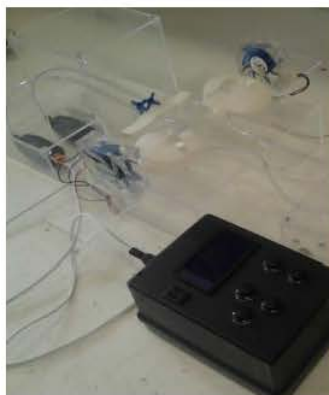
Figure 2. Phantom for dynamic renal scintigraphy.
